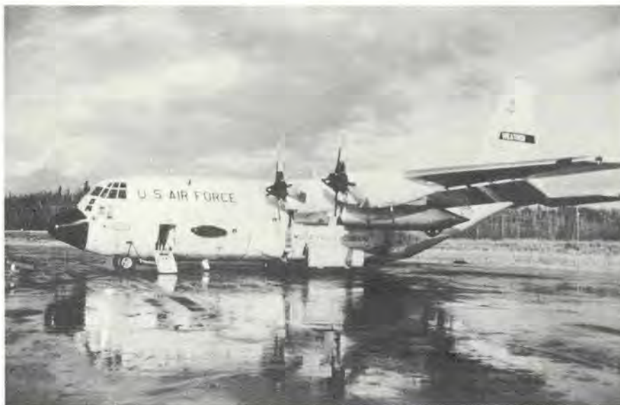
Fig. 1 An AWS WC-130 Hercules, specially equipped with an airborne dry ice crusher and dispensing system, was used this past season in projects to dissipate supercooled fog at Elmendorf AFB, Alaska, and Hahn, Bitburg and Spangdahlem Airbases in Germany.
