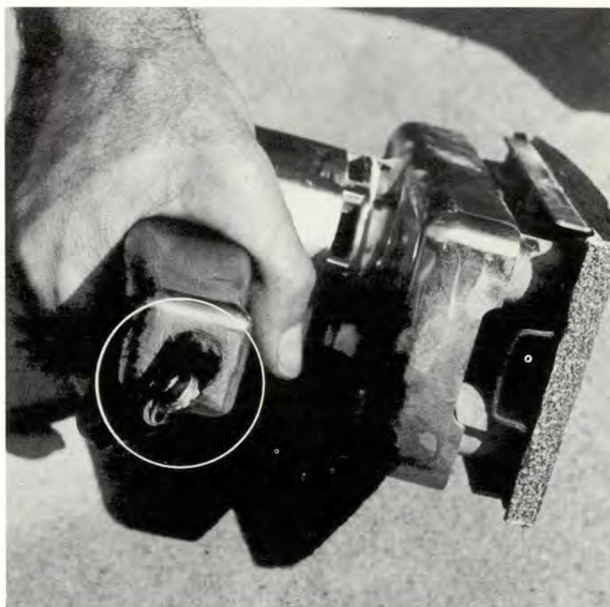
Lifting tool by the cord and other abuse will eventually break the lead-in fitting. Replace the cord before it shorts and ignites sanding dust! Dust can explode with considerable force.
